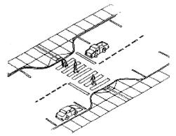
Figure 3 – Example of a Curb Extension
