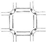
Figure 2 -- Conventional Crosswalk Markings
